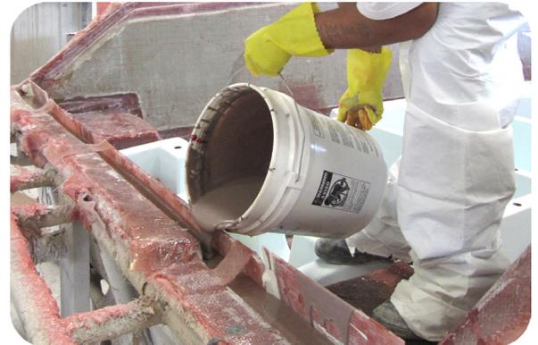
**ABOVE:** Pouring Arjay CPC into cavity between special FRP laminate and hull transom laminate
